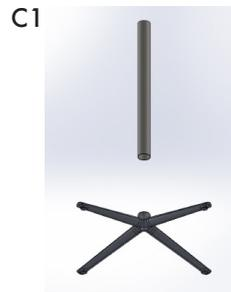
4. Remove the glides from the base using a flat head screw driver if necessary.
